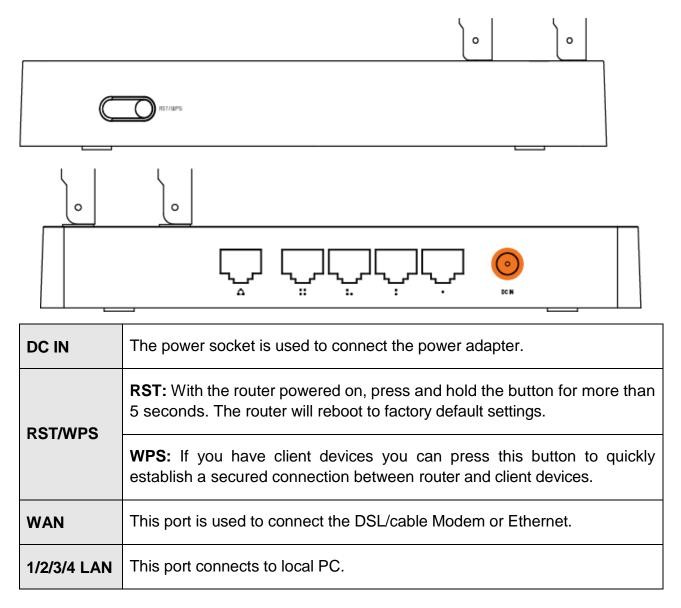
**Note:** Press and hold RST/WPS button for less than 5 seconds, the router will enable WPS function. Press and hold WPS/RST button for more than 5 seconds, the router will enable RESET function
